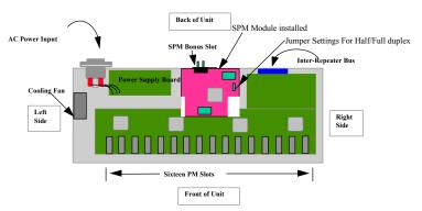
Fig. 3.10.1a Top View: SPM Module Installed in a 8000X
